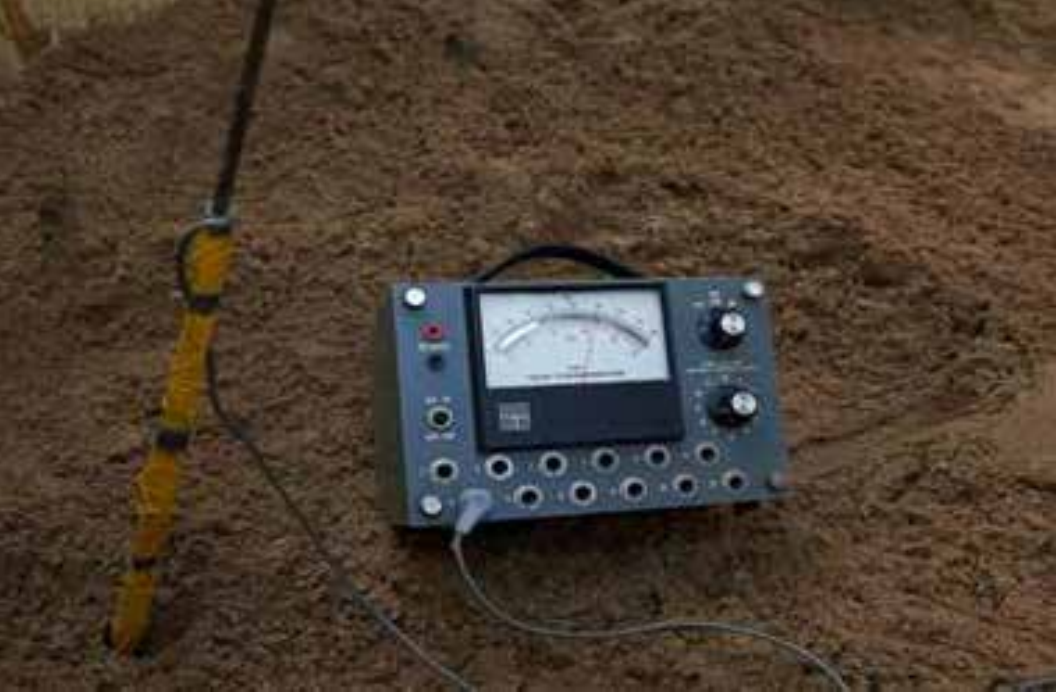
FIGURE 8: INSERTION OF TEMPERATURE PROBE AT SPECIFIC DEPTH TO DELINEATE TEMPERATURE GRADIENT. PHOTO: JULIE MAHER©WCS
