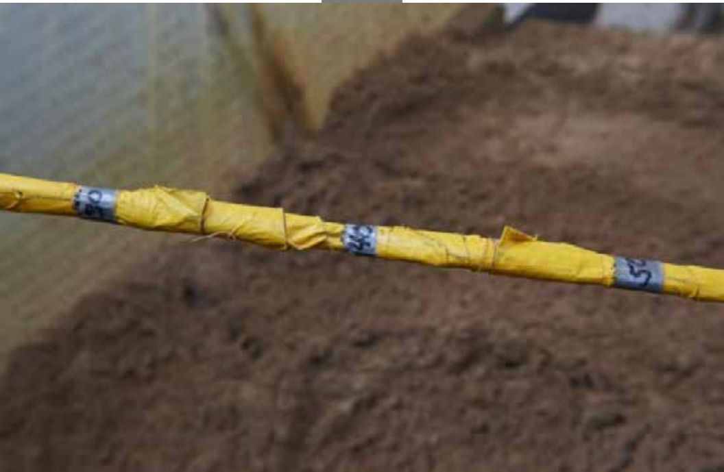
FIGURE 6: TEMPERATURE PROBE WITH DEPTH CALIBRATIONS. PHOTO: JULIE MAHER©WCS
